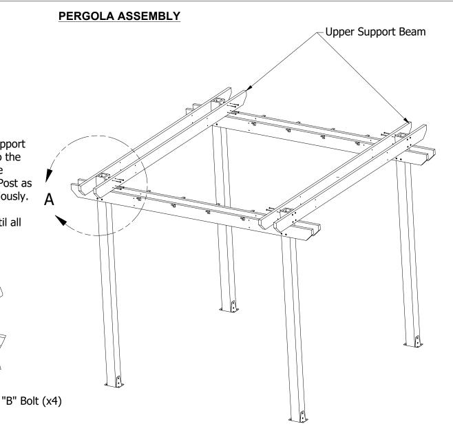
**15)** Attach the Remaining (2) Upper Support Beams Using (16) "B" Bolts, as Shown to the Right and in Detail "A". These Should be Installed on the Opposite Sides of Each Post as the Upper Support Beams Installed Previously.
