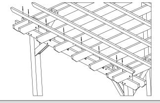
**32)** Secure Each Remaining Top Slat with (7) "D" Screws.
