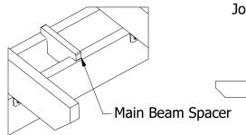
**24)** Place the Main Beam Spacer Between the Lower Support Beams as Shown Above to Maintain the Correct Beam Spacing.
