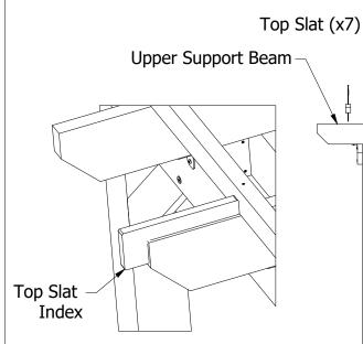
**29)** Use the Top Slat Index to Set the Location of the First Top Slat. Set the Top Slat Index on Top of the Joist as Shown Above, and Adust the Top Slat Until it Rests Against the Top Slat Index.
